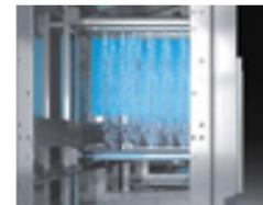
M-iQ employs a high-pressure wash for improved soil removal and reduced water consumption. Water flow has been modeled using computational fluid dynamics. Water, energy and chemical consumptions are all dramatically reduced.
